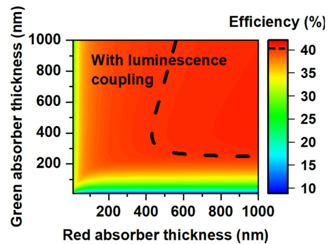
We calculated the maximum efficiency with different thicknesses of the two (red and green) halide perovskite layers. The dashed line shows the thicknesses needed to get 41% efficiency.
