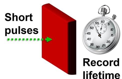
We needed to understand how halide perovskites could lose the energy absorbed from the sun. To do this we fired short pulses of light (like camera flashes) at the halide perovskite and timed how long the absorbed energy lasted within the material.
