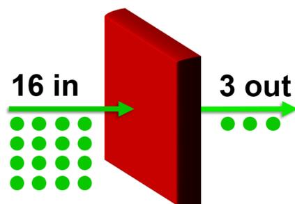
We measured the amount of light each halide perovskite could absorb. We sent a known number of photons (light particles) at the halide perovskite and counted how many were not absorbed. In this example 13 out of every 16 photons are absorbed.
