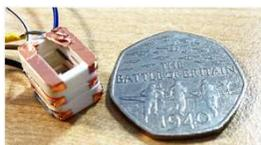
The coin-size 3D printed breath analyzer could **identify the pattern of breath leakage through face coverings and detect cough sound**. We found most leakage from surgical masks comes from the front; while most leakage from N95 masks comes from the sides with tight fittings.
