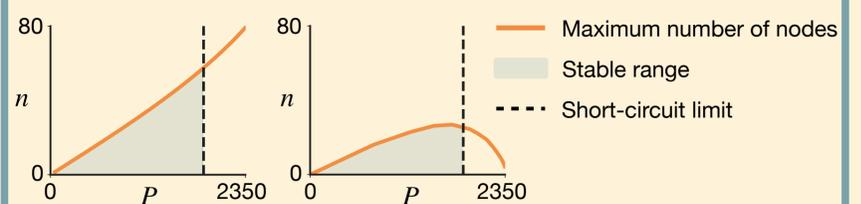
The control system on the left has a large stable regime and would be **capable of providing a power grid with nearly 100% renewables**, whereas the control scheme on the right has a small stable regime and would fail.
