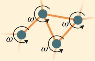
These rotating machines must supply the UK grid with AC power at a uniform grid frequency  $\omega$  of **50Hz** and a **constant voltage of 240V**. The grid's **stability** is its ability to maintain these values.
