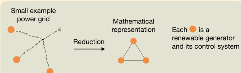
This way, large complex power grids can be represented as simpler structures. The stability of this reduced network is then assessed by formulating the system's Master Stability Function<sup>[3]</sup>.
