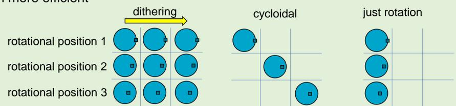
Cycloidal CT uses only a fraction of the data compared to dithering: it's **faster** and it delivers **less dose**. It uses the same amount of data as just rotation, but it spreads it in a smart pattern to improve quality.
