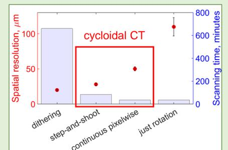
The spatial resolution of cycloidal images is very close to that of dithering, while taking up to 20x less time. Just rotation, which takes the same amount of time, has much worse resolution.
