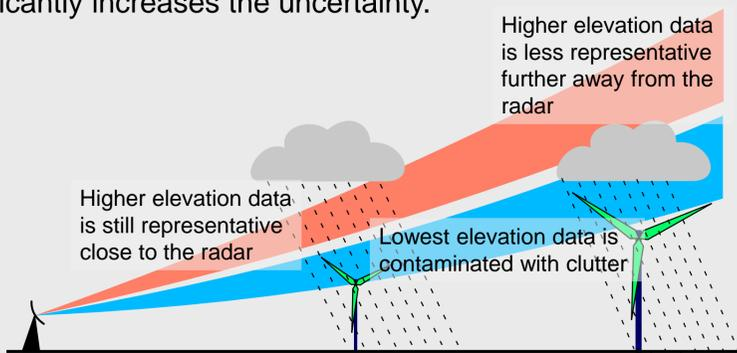
Figure 1. If a small turbine is found close to the radar, a higher altitude measurement may be sufficient to estimate the surface rainfall. Further away from the radar, the higher altitude measurement may not be representative of the surface rainfall. (not to scale)
