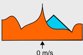
Figure 3. Unlike ground clutter, the signal from a wind turbine field has significant multimodal non-zero velocity components.
