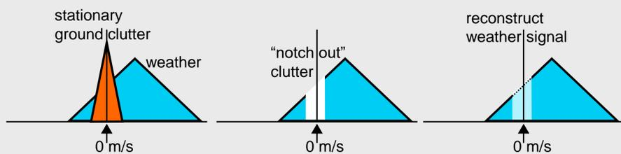
Figure 2. Ground clutter (zero radial velocity) signal can be removed from the measurement and the original weather signal can be reconstructed.
