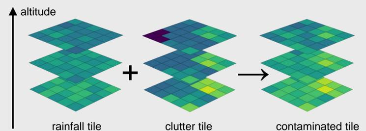
Figure 4. Rainfall and clutter signals at multiple altitudes are systematically combined to produce contaminated tiles with a known ground-truth.
