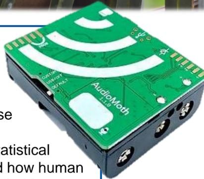
Fig. 1. AudioMoth acoustic recorder
