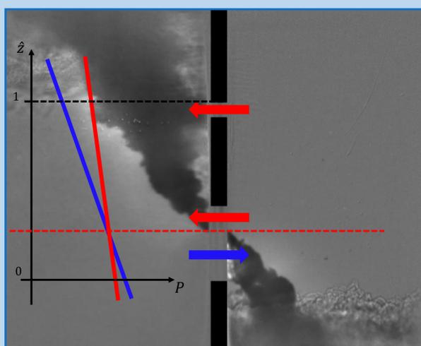
Fig 3. Shadowgraph of a water tank experiment for an asymmetric geometry. A bidirectional flow is observed in the lower opening, with light fluid flowing into the left tank and dense fluid flowing into the right tank. Pressure profiles are plotted as references.
