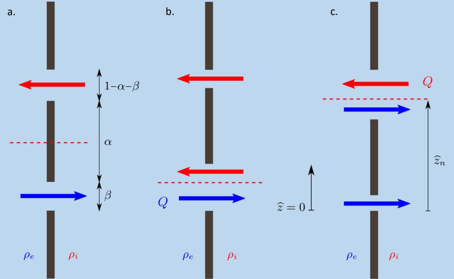
Fig 1. A traditional sash window has two sliding panes allowing the window to be open at the top and/or bottom. Depending on the geometry, the relative position of the neutral level will vary and different flow regimes appear: (a) unidirectional flow, (b) bidirectional flow at the lower opening and (c) bidirectional flow at the upper opening.
