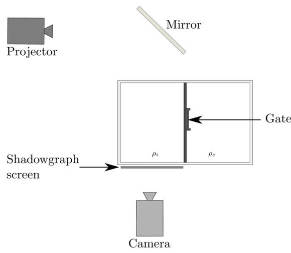
Fig 2. Schematic of the experiment with a top view of the tank divided into two compartments. The sash window opening is closed by the vertically-sliding gate.
