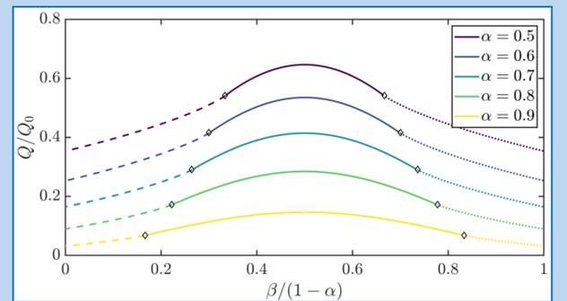
Fig 5. Variation of the flow rate, normalised by the flow rate of an open rectangular window of dimension  $W \times H$ , with the height of the lower opening.  $\diamond$ : transition from one regime to another.
