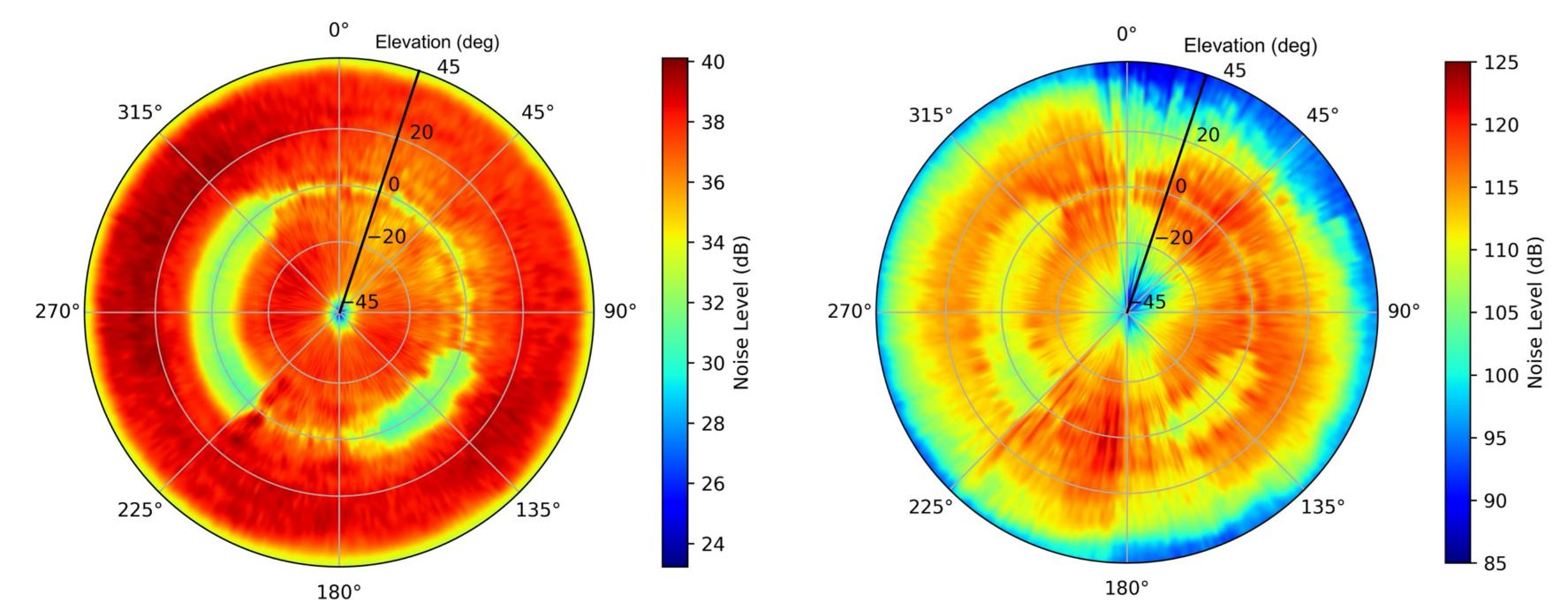
Directional Ambient Noise Intensity in elevation and bearing at 55Hz for **wind**.
