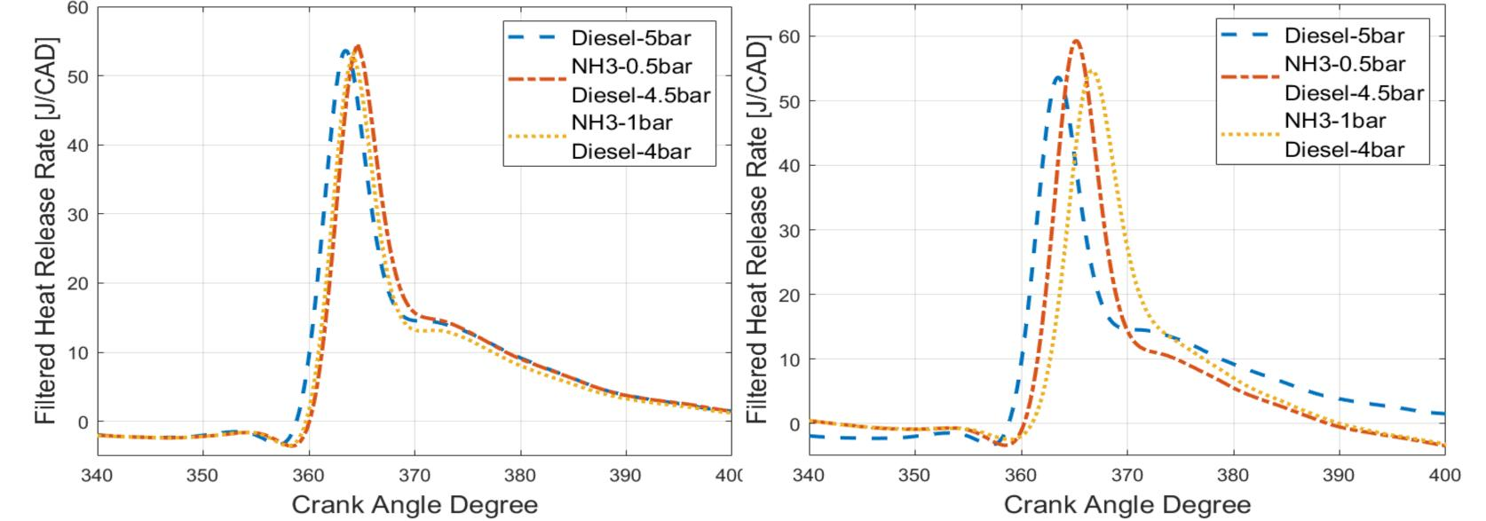
• NH<sub>4</sub>NO<sub>3</sub> does not significantly change the peak heat release rate • 0.5 % NH<sub>4</sub>NO<sub>3</sub> offsets the increases in delay of combustion observed with an increasing contribution of aqueous ammonia to engine load
