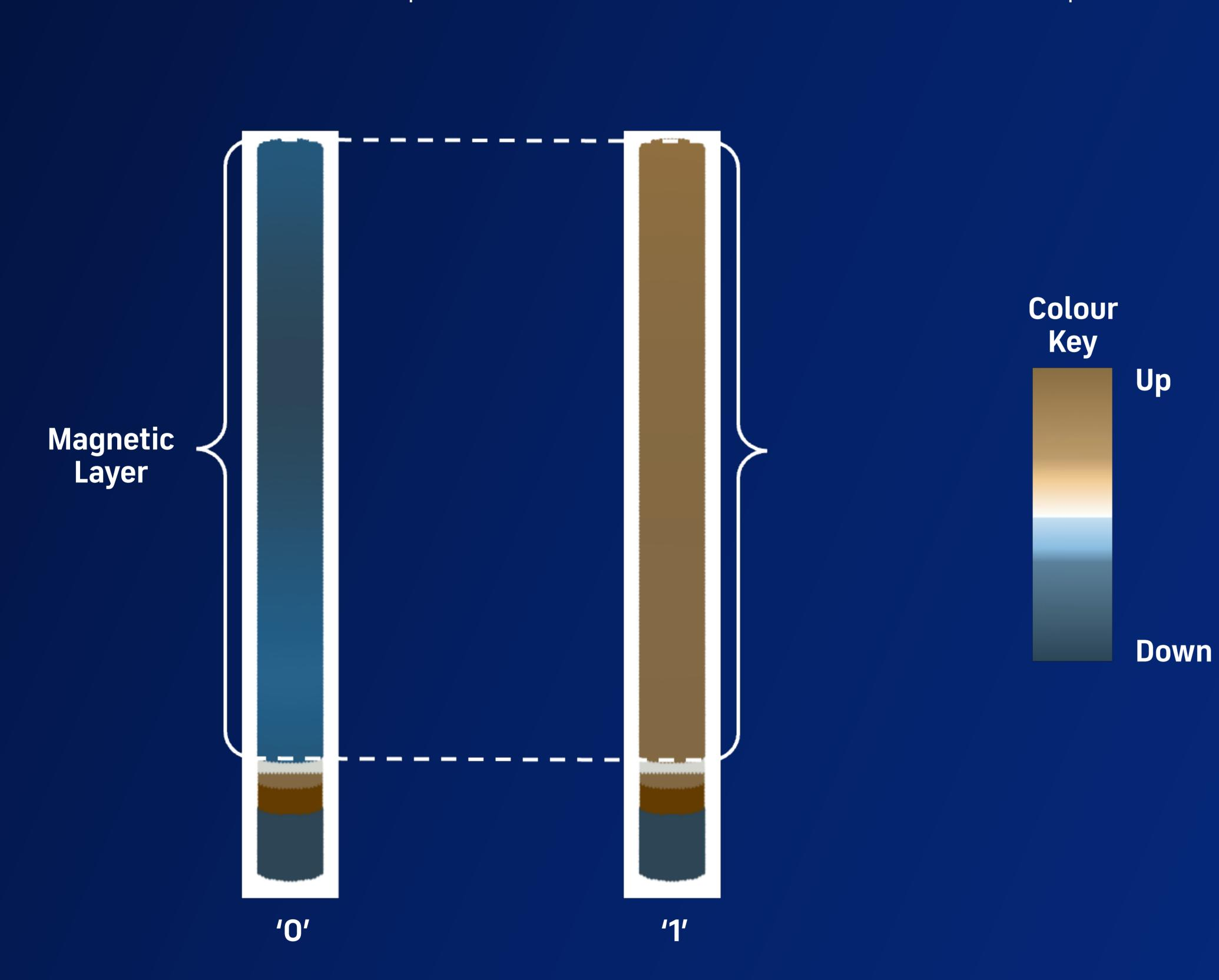
Magnetic RAM consists of a magnetic layer, which can align up '1', or down '0'. It is reversed via a '**reversal** current'. Once a magnetic state is saved, it draws no further power (non-volatile).
