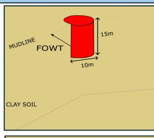
MUDLINE FOWT1 FOWT3 15m FOWT2 With a shared anchor, the diameter of the caisson anchor supporting three(3) 15MW offshore wind turbines **was reduced by 25%, reducing CO2 emissions** compared to when a single caisson anchor was used to support one 15MW offshore wind turbine.
