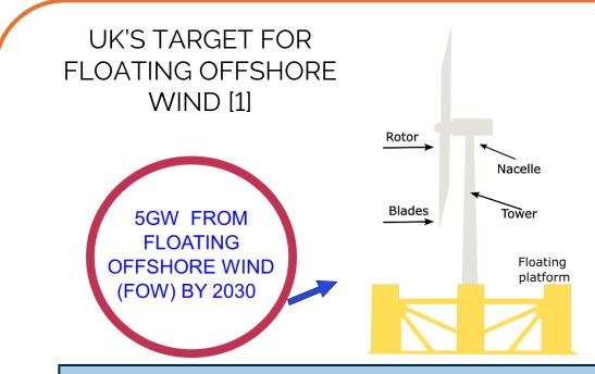
To meet the UK's target, Offshore wind turbines are moving into deeper waters to harness more energy from wind.
