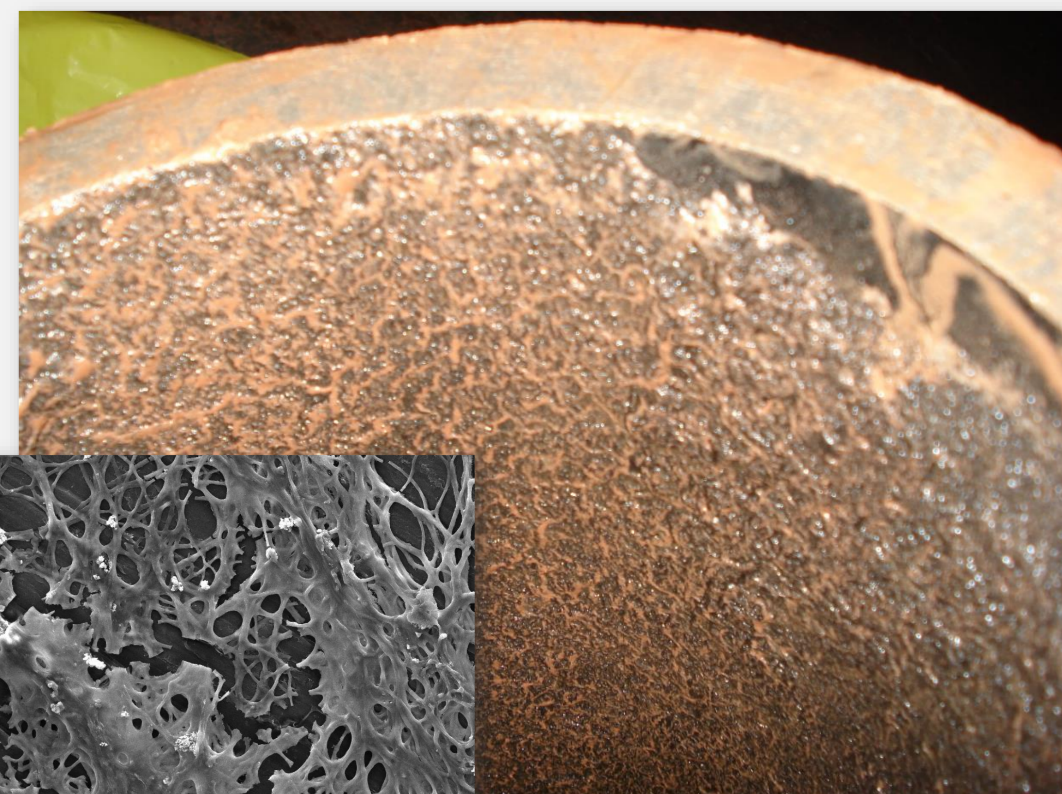
Photograph and scanning electron microscope image of drinking water biofilms.
