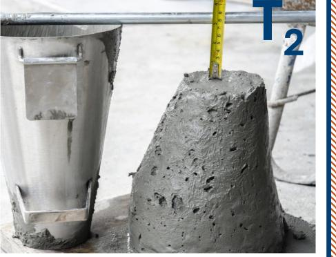
The slump test is conducted on almost every UK construction site. Currently, a ruler crudely measures how much the concrete falls when a mould is removed.
