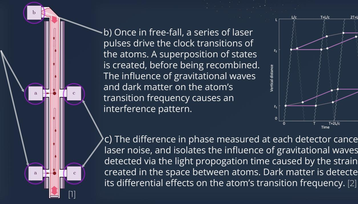
b) Once in free-fall, a series of laser pulses drive the clock transitions of the atoms. A superposition of states is created, before being recombined. The influence of gravitational waves and dark matter on the atom's transition frequency causes an interference pattern.
