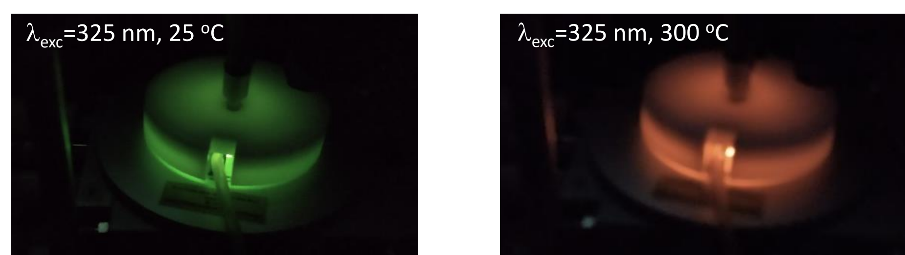
Photographs of the MOF powder under irradiation of UV light at different temperatures in air. The image on the left was taken at 25 °C where the MOF emits a green colour and at 300 °C where the MOF emits an orange/red colour.
