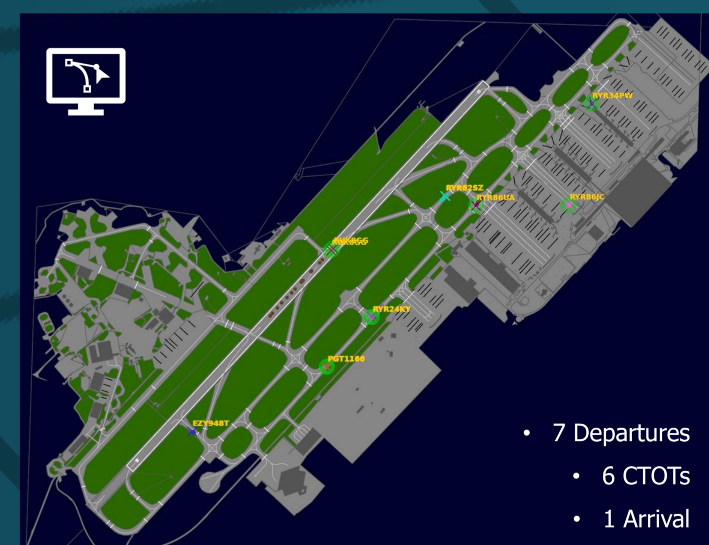
Fig. 4 Air Traffic Control Airport Radar (ASMGCS) used to visualize Futuristic Air Traffic Control's airport management.
