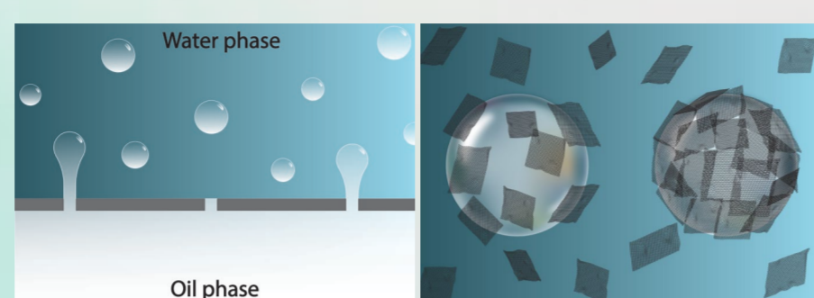
Fig. 2. Fabrication of graphene-coated silicone droplets.
