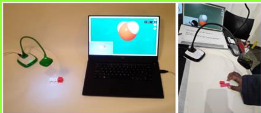
Left: the app detects 2 white blocks and 1 red together, and displays a spinning H 2 O molecule. Right: Modelling a simplified carbohydrate molecule with Cuisenaire rods
