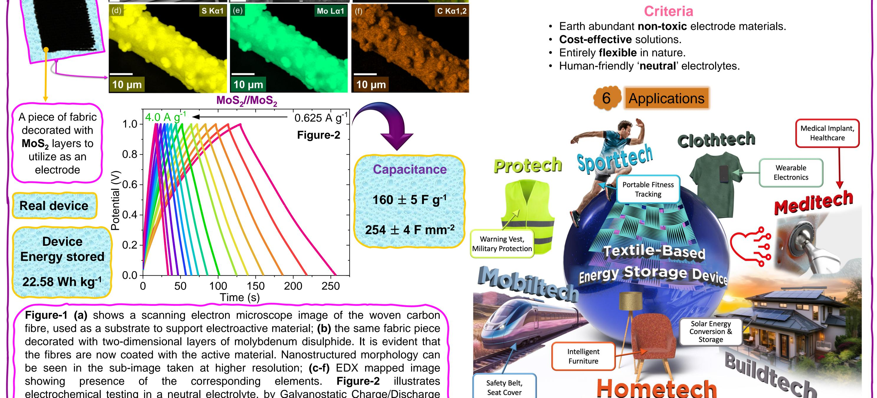
be seen in the sub-image taken at higher resolution; (c-f) EDX mapped image showing presence of the corresponding elements. Figure-2 illustrates electrochemical testing in a neutral electrolyte, by Galvanostatic Charge/Discharge which quantifies the charge stored by the electroactive material. This result indicates that the device possessed a capacitance of 160 F/g, which is highly promising explicitly for small scale applications. ReNU 🖧 👖
