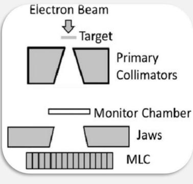
A linac head is made up of heavy material (e.g. tungsten and lead) used to shape the radiation beam. There are fixed shielding parts such as a "primary collimator" and dynamic shielding parts such as "jaws" and a "multi leaf collimator". To simulate the effectiveness of the treatment head's radiation shielding, 3 billion, 6 MeV incident electrons were simulated using the Monte Carlo method.
