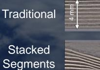
Through-thickness reinforcement is achieved which reduces spread of delamination damage
