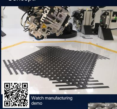
Using tape-by-tape manufacturing, split plies into segments of alternating tapes
